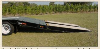
Standard 8'x3' hydraulic ramps with electric over hydraulic power unit makes loading fast and easy.
