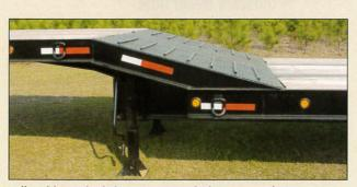
Full width gradual slope to upper deck means utilizing upper deck space for loading.
