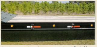
9 "D" rings per side, mid span turn signals, and flag holders as standard equipment.
