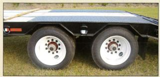
Hutch 9700 Spring suspension ● 255/70R 22.5 (H) Low profile steel belted radials ● Outboard mounted oil bath hubs ● 10-Hole Budd wheels
