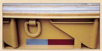
9 Heavy Duty "D" Rings per side • Load bearing outriggers - spaced every 24".
