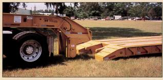
Non-Ground Bearing Neck w/self-contained pony motor. Selfaligning neck for easy detaching.
