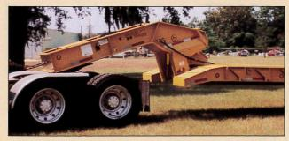
Adjustable ride heights eliminates problems with crossing railroad tracks, loading (unloading) on soft ground and getting into job sites.
